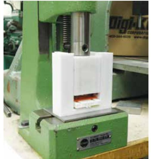
Thogus Products is an injection molder that specializes in low-volume manufacturing and highly engineered materials. By 3D printing their factory-floor tooling instead of outsourcing, Thogus achieves dramatic cost savings. In one particular example, Thogus produced a 3D printed CMM fixture overnight, saving 70-90% on lead time compared with outsourcing.
